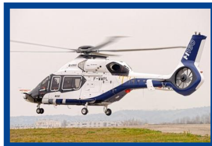
First flight of Arrano 1A on Airbus H160
