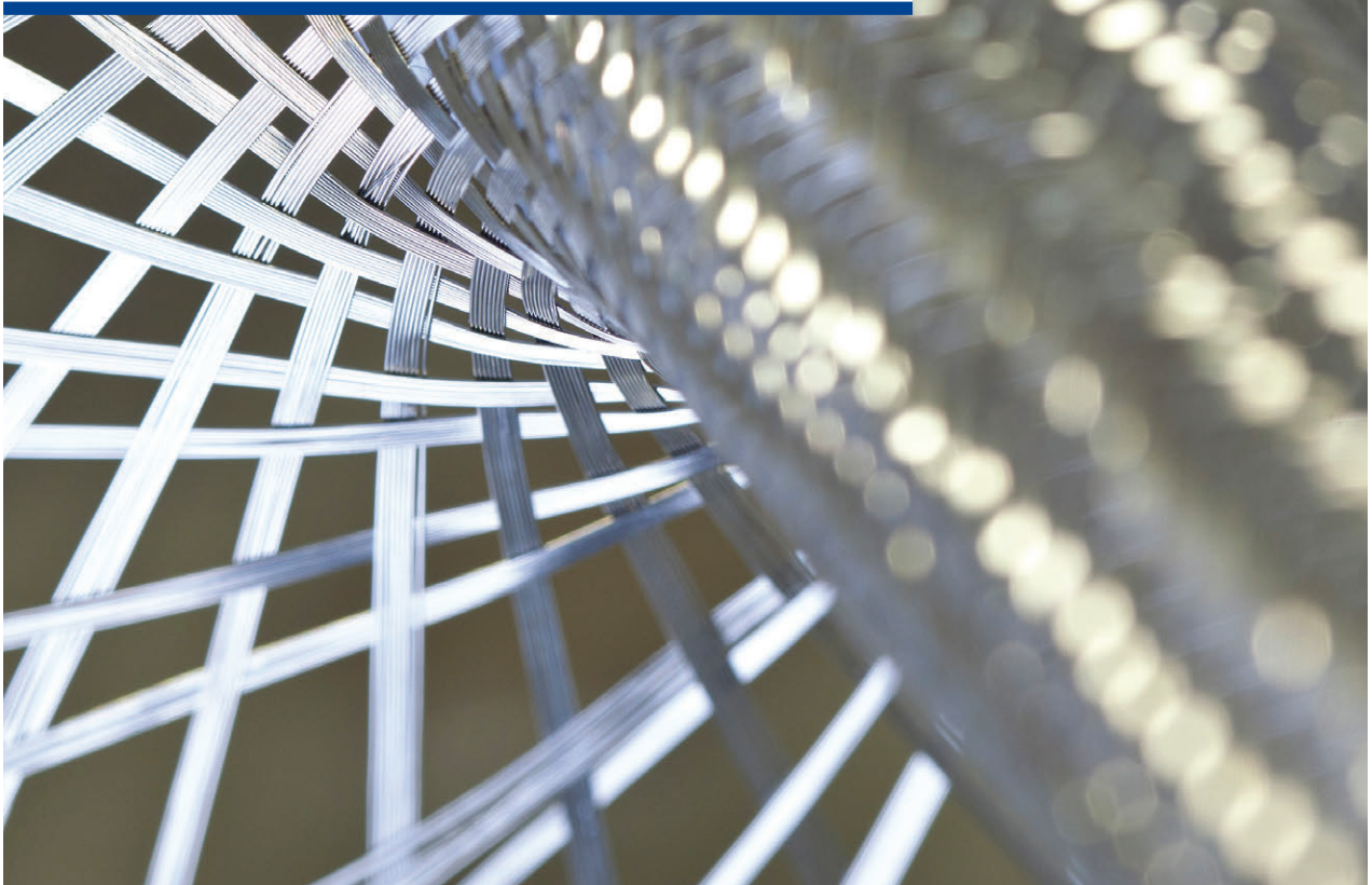
Protective overbraiding of an aerospace harness
